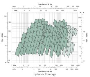
that will meet the original specifications and expected variation and degradation of the flow system. The picture above is a Gould Pump Selection chart. Each of the "tombstones" represents a particular pump model and its flow-head relationship. This chart helps the manufacturer's salesperson narrow the search for a particular pump model/style/size.
