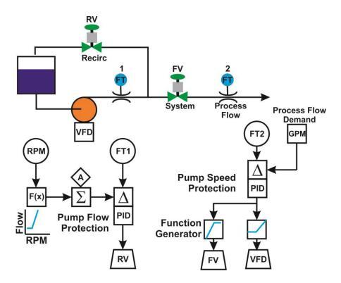
In this arrangement the minimum flow would follow the RPM (or frequency)/flow chart down until it reached a minimum flow setting. At that setting the recirculation valve (RV) would begin modulating to maintain the minimum flow through the pump (FT1). The operator is provided with a BIAS in the control scheme to provide additional flow margin if necessary.
