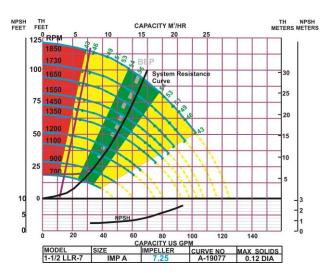
chart we will use 20 feet of head as the minimum pressure across the pump and at that head 15 GPM is the pump flow protection. We can see that the system resistance will need to be modified with a flow valve to compensate for the pump's inability to control below 20 feet of head.
