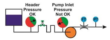
The reason the "inlet of the pump" is capitalized and underlined in the first paragraph of this section is that using pressure measurements in the piping upstream of the pump suction is not acceptable. Many times the process designers do not account for the piping pressure losses, restrictions or adverse dynamics between the inlet header and the pump inlet. The resulting pressure, Net Positive Suction Head Available (NPSHA), at the inlet falls below the NPSHR.
