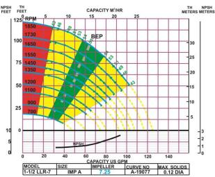
slightly. The red area still represents a do-not-operate in this region. However you will note that it decreases as function of RPM. We need to respect the NPSH for the pump since the velocities at the inlet of the pump are still related to the flow at the inlet eye of the impeller.
