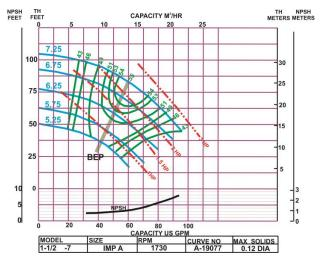
1730 RPM. (This data represents a 4-pole induction motor with an unloaded speed of 1800 RPM). There is a 70 RPM slip between the line and motor shaft while under load. This chart is not immediately useful to the engineers since we need to view only one impeller size (7.25 inch) at multiple speeds.
