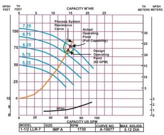
or exceed the requirements of the process system. As noted above, we have selected the 7.25 inch impeller which exceeds the design operating flow.
