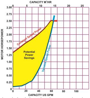
The variable speed power usage does indeed show that the system has the opportunity to save significant power. If the system normally runs at the 60+ GPM point, then the savings will be minimal. A detailed analysis of the costs and small benefits should then be carefully weighed. If the system operates
