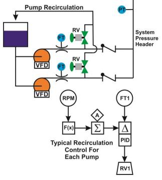
flow on one pump while the other pump may require significant protection. For this application it may be necessary to provide a flow-balancing arrangement for the pump flow.
