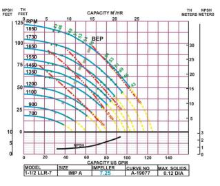
on the new speed curve. This may appear to be a laborious task, but a computer and spreadsheet can make the task more manageable. Each pump speed must be calculated in a similar fashion and plotted to create a new set of pump curves applicable to a VFD application.
